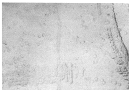
Figure 4 Etch pattern formed by 6.6 N citric acid at 51° C after 1 h 10 min, × 150.
